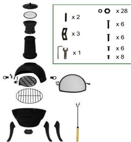
1. Screw feet on with 6x x-large screws
