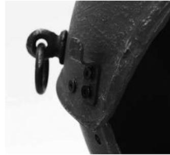
6. Attach handles on with 2x special screws
