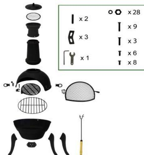
1. Attach feet with 6x x-large screws
