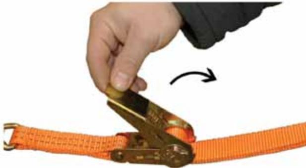
Secure the strap to the ground by pushing the peg through the metal hook. Tension the strap by lifting the ratchet up and down.
