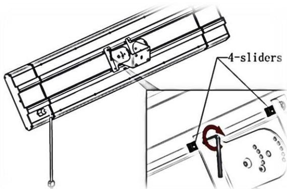
**Step 3:** Fix the part 1 ① on the wall, tighten the four nuts (a part of explosive bolt M6\*50) ② with M6 spanner ⑪.
