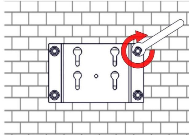
**Step 4:** Put the heater on the wall, slide it into the part 1 ①.
