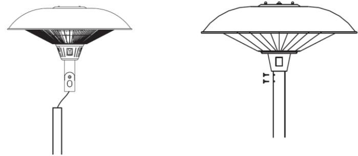
Step 7: Raise or retract the top pole to the desired height and tighten to the middle pole by screwing knob down.
