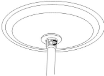
Step 10: Connect the upper pole with middle pole by screwing them together.
