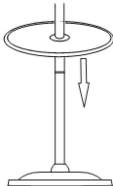
Step 5: Place the power cord plug through base, bottom pole, middle pole, Connect the power cord plug to the socket in the heater head.
