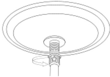
Step 9: Tighten the Plastic Fixation Part by screwing the Screw Knob.
