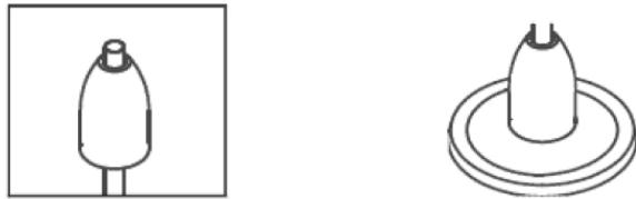
Step 3: Connect the middle Pole with bottom pole by screwing them together.
