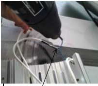
19 Fourteenth step: blow the black silicone tube tightly with hotblower.
