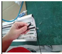
16 Eleventh step: set the opposite end wires into black silicon.
