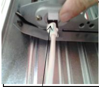
7 Third step: fix the heating element with connection cable.
