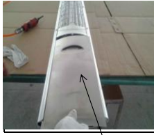
2 Second step:pull PCB protection board out.
