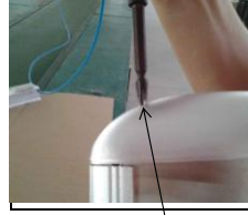
8 Eighth step:remove the screw of the aluminium cover.
