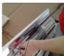
24 Twenty-second step:pull the heating element 1 out.
