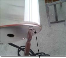
1 First step:remove the screw of the under damper.
