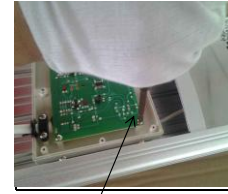
5 Fifth step:remove the screw of the PCB board.
