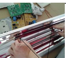
22 Twentieth step:two hands hold the heating element clamp.
