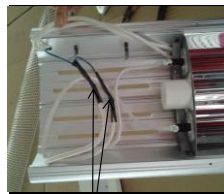
13 Thirteenth step:pull the two wires to see black silicone.
