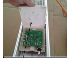
4 Fourth step:open the PCB box top cover .
