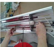
26 Twenty-third step:repeat nineteenth,twentieth,twenty-first step,pull the heating element 2 out.
