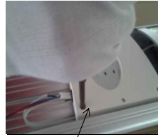
3 Third step:remove screws of the PCB box top cover.
