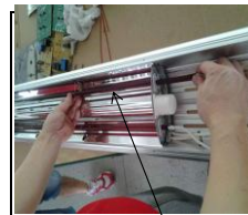
23 Twenty-first step:pull the heating element 1 out.
