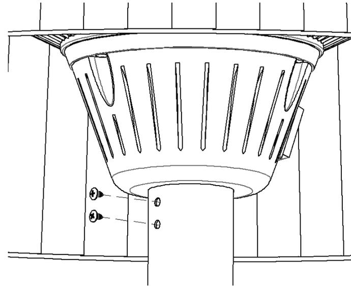
Step 6: Fix the Power Cord on the Base by using 4\*12mm screws.
