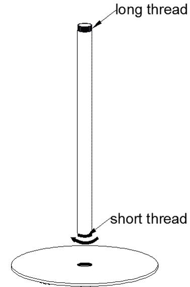
Step 2: Connect the middle tube with bottom tube by screwing them together.
